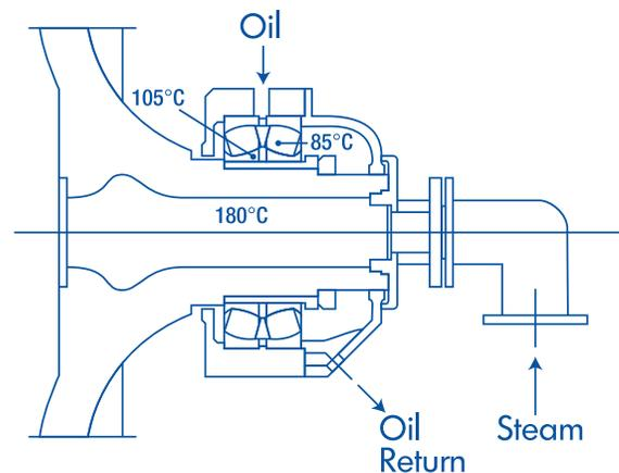
➔ Steam is passed through the cylinder to heat it. The journal expands faster than the bearing, making the fit tighter. Severe hoop stress on inner ring is repeated every time the machine is started. Inner ring fracture is a common problem.
